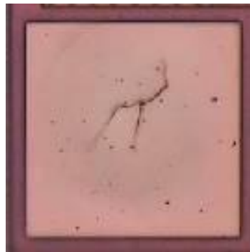
Crack is visible on pad surface
